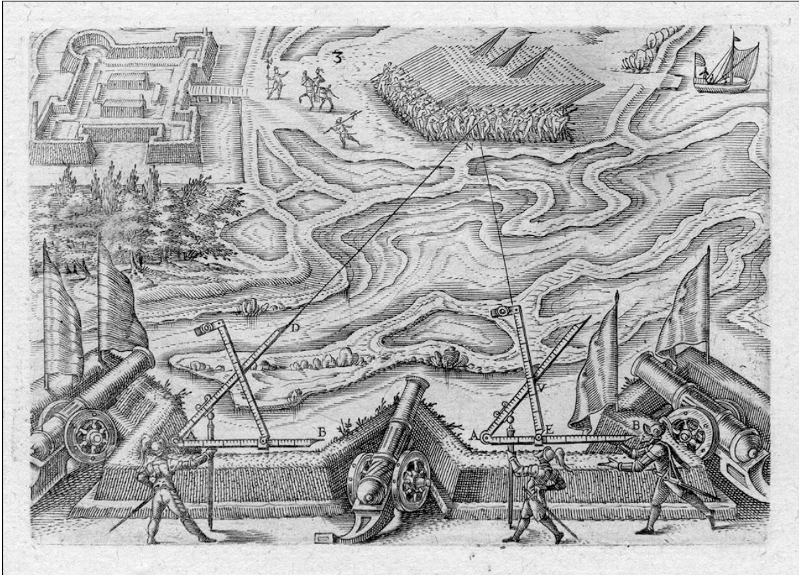
Figure 1.4: Jobst Bürgi's triangulation instrument used to determine the distance of enemy troops, before firing cannon, published in Kassel/Germany, 1648.
